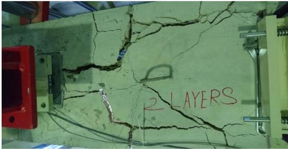
Figure 14 Diagonal cracks in the flange from the experimental program – top view
